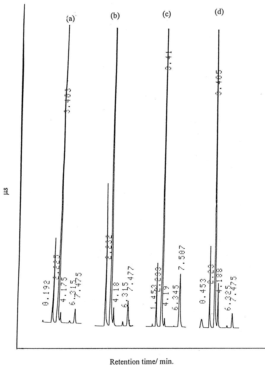
Fig. 2. Chromatogram of nitrate and nitrite of human saliva, with suppressed conductivity detection. (a) Unspiked saliva; (b) unspiked saliva; (c) spiked with nitrate (2 \mu\text{g}/\text{ml} ); (d) spiked with nitrite (2 \mu\text{g}/\text{ml} ). Nitrite retention time=4.1 min and nitrate retention time=7.5 min. Other conditions as in Fig. 1.
